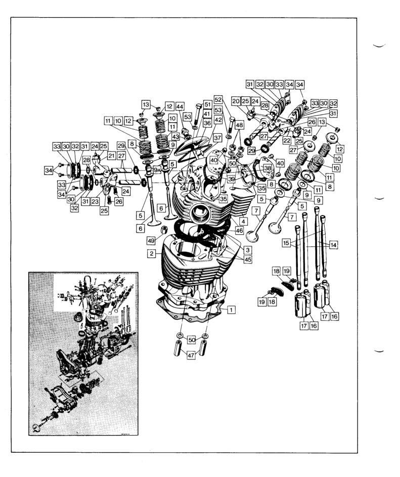
**Engine: Cylinder, Cylinder Head and Fittings**
