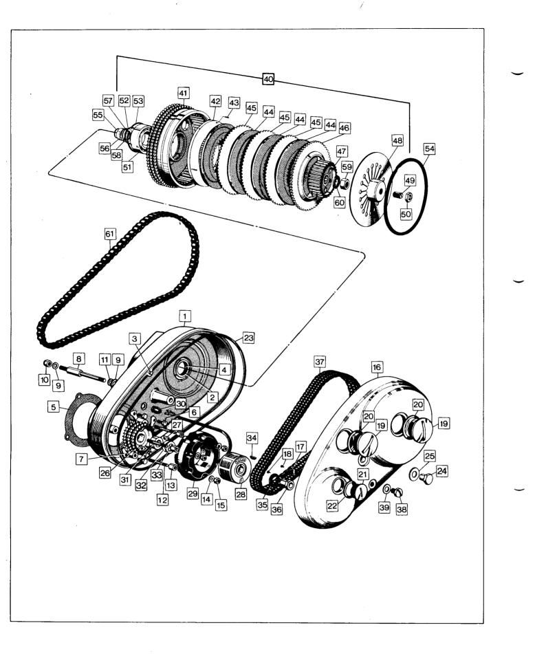
Chaincases, Chains, Sprockets, Clutch, Alternator
