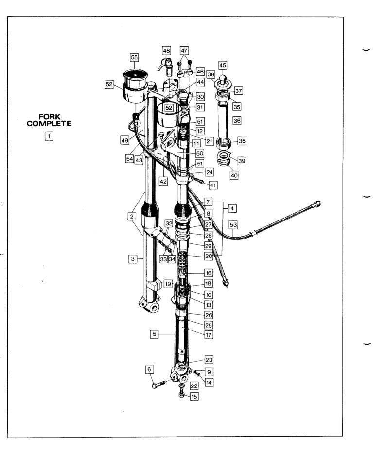
Front Forks, Steering Lock, Steering Head Bearing, Tachometer, Instument Cases
