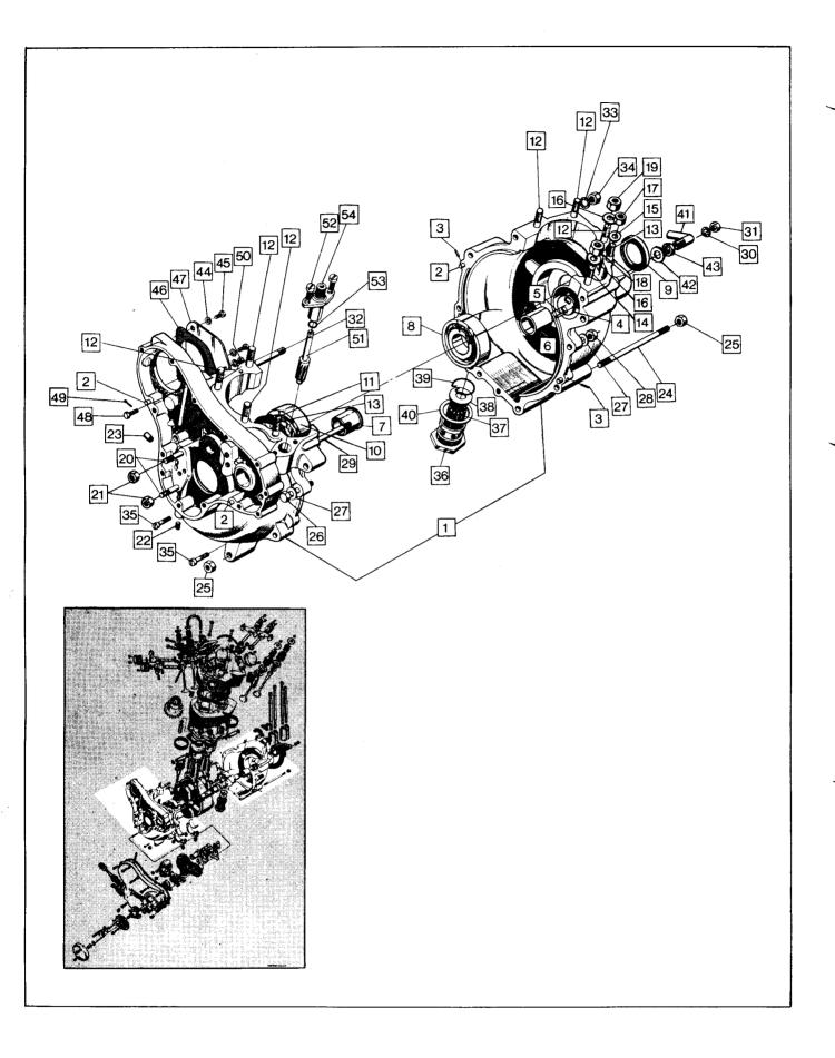
Engine: Crankcases, Crankcase Filter, Tachometer Drive
