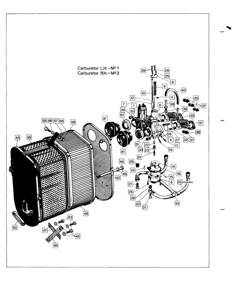
Carburetors, Fuel Lines, Air Filter, Carburetor Mountings
